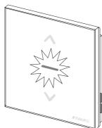
**5\***. Programming error – button flashing for 2-3 sec. as presented in the drawing.
