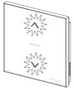
**5\***. Programming error – buttons flashing for 2-3 sec. as presented in the drawing.
