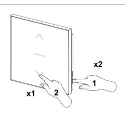
1. Press within 1.5 sec. In/Ex button twice (1) and once operating readiness for device deleting button "down" or "up" (2)
