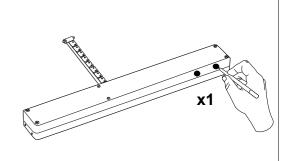
**3**. Press "P" button on the device and hold it for 0.5 sec. (see Device Programming Manual).
