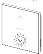
**5\***. Programming error – button flashing for 10 sec. as presented in the drawing.
