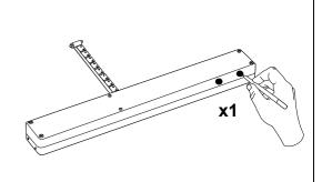
3. Press "P" button on the device and hold it for 0.5 sec. (see Installation Manual).
